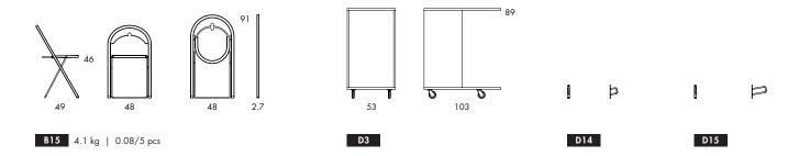
**FOLDING CHAIR**. Back and seat arc in compression moulded, layer-glued, clear-lacquered birch veneer. Seat and back in lacquered birch. Legs in chrome-plated (chrome III) or black-painted steel.
